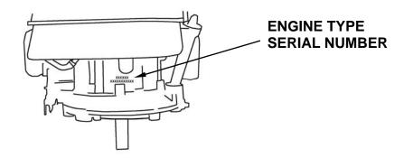
Record the engine serial number in the space below. You will need this serial number when ordering parts, and when making technical or warranty inquires.
